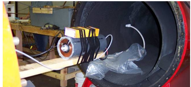
Fig. 6. Helical flux compression generator ready to be placed into the explosive chamber.
